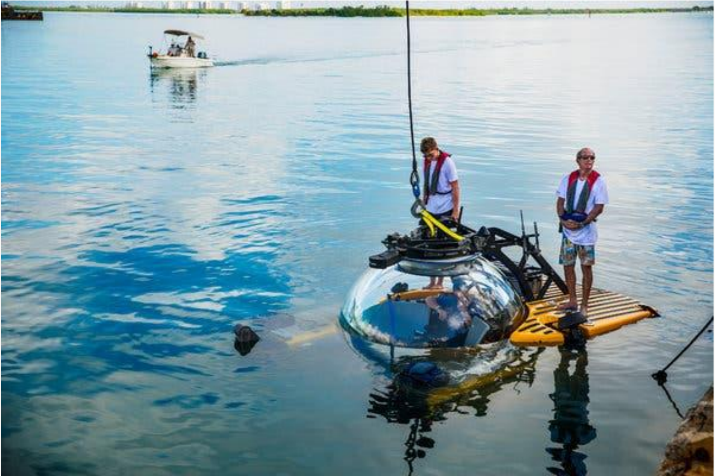
A Triton 3300/3 submarine during a surface stability test by Triton technicians and engineers in Fort Pierce, Fla., in October. Scott McIntyre for The New York Times
